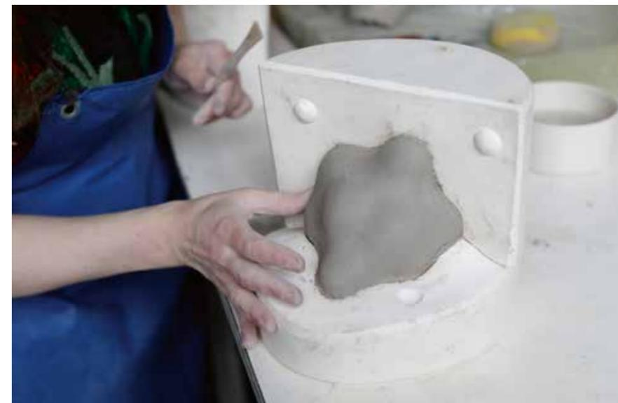
**8** I then gently lift off the mould and clean the joins. I use the excess clay that has been pressed out from the mould to blend back into the join to reinforce it. The edge around the mould here shows where I have done this. A wooden tool is helpful at this stage. Fettleing is done once the parts are removed from the mould.
