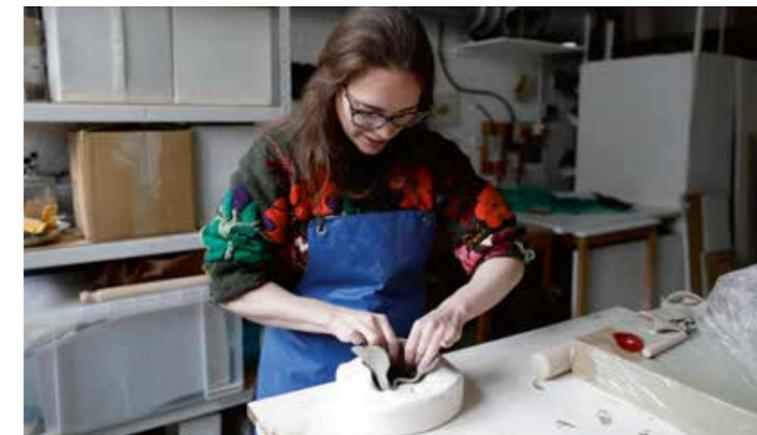
**4** I fit the clay into the mould, easing it in gently from the sides and the top, rather than pushing the clay down in the middle. This way the clay is not pushed too thin and remains an even thickness. Problems can occur in the firing if the parts in the mould are of different thicknesses, as any discrepancy means that heating and cooling take place at dissimilar rates, which causes cracking.
